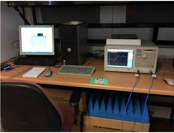
Fig. 4. Experimental set-up (PC with LabVIEW and VNA).
